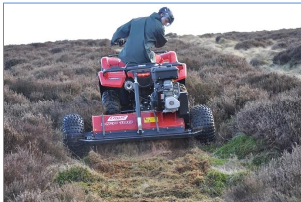
Figure 10 – Quad bike and self-powered flail mower
