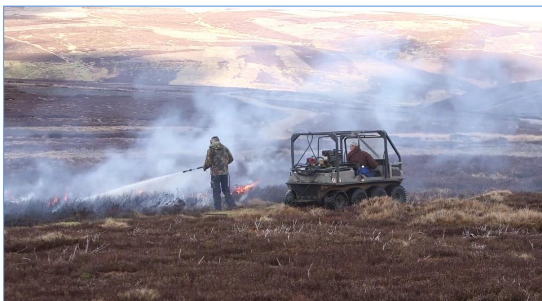
Figure 7 – Vehicle-mounted fire fogging equipment
