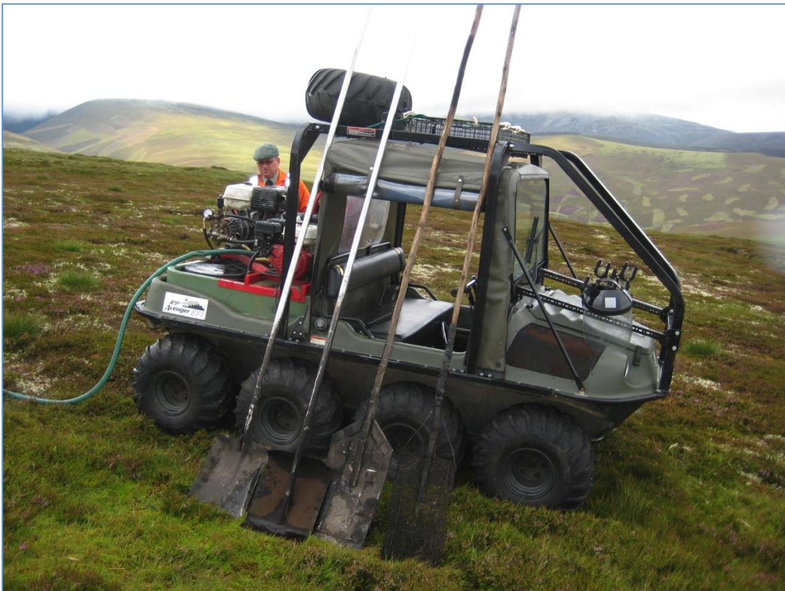
Figure 11 – All Terrain Vehicle, with fire-fogger and fire beaters
